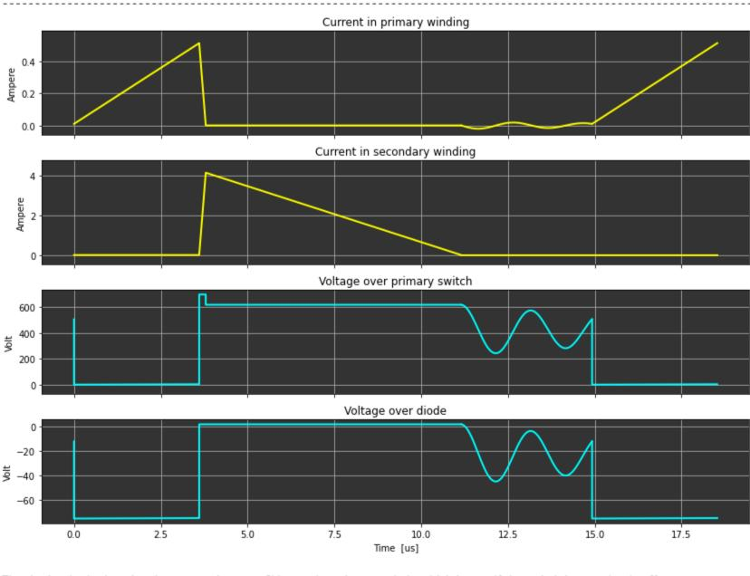
The ringing in the inactive time can swing to < 0V over the primary switch, which is true if the switch is completely off.
